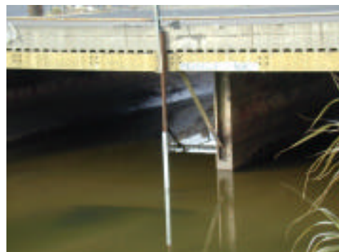
Picture 1: Staff gage measuring water level
