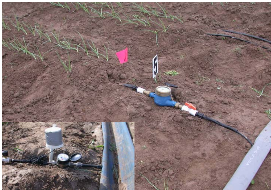
This photo provides a close-up view of economical totalizing water meters that were installed to record water inputs on onion fields. At each site, a sensor (inset) was installed to record irrigation data
