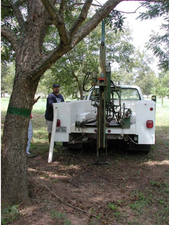
PVC pipes were installed using the soil coring truck to facilitate the use of neutron probes to monitor water conditions.
