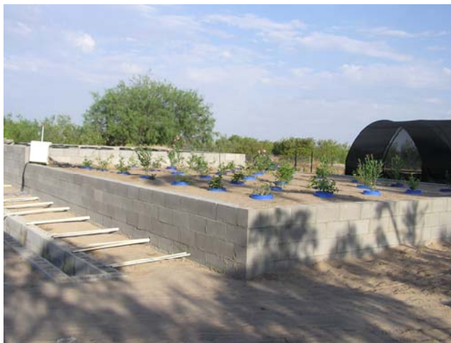
Lysimeters have been constructed in El Paso to determine plant water use.
