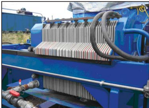
Fig. 2: EC Unit with Iron Electrodes Built on a Filter Press Frame
