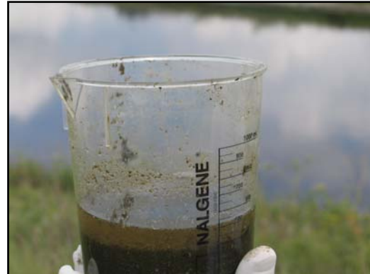
Dairy effluent reacts with alum and polyacrylamide polymer and as a result, separates into solid and liquid layer.
