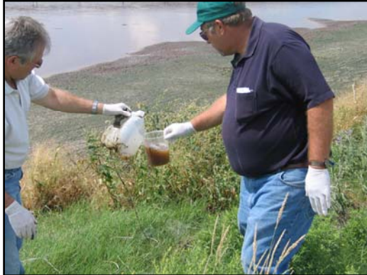
Geotube personnel mix dairy effluent with experimental ratios of alum and polyacrylamide polymer to bind with P in effluent.
