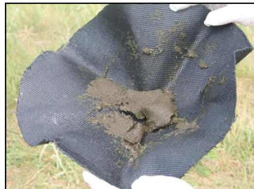
Residual solids within Geotube ® material following filtration and P binding.
