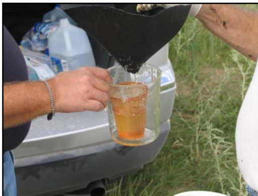
Dairy effluent mixture filtered through Geotube ® material and filtered water collected to determine amount of P reduction achieved.
