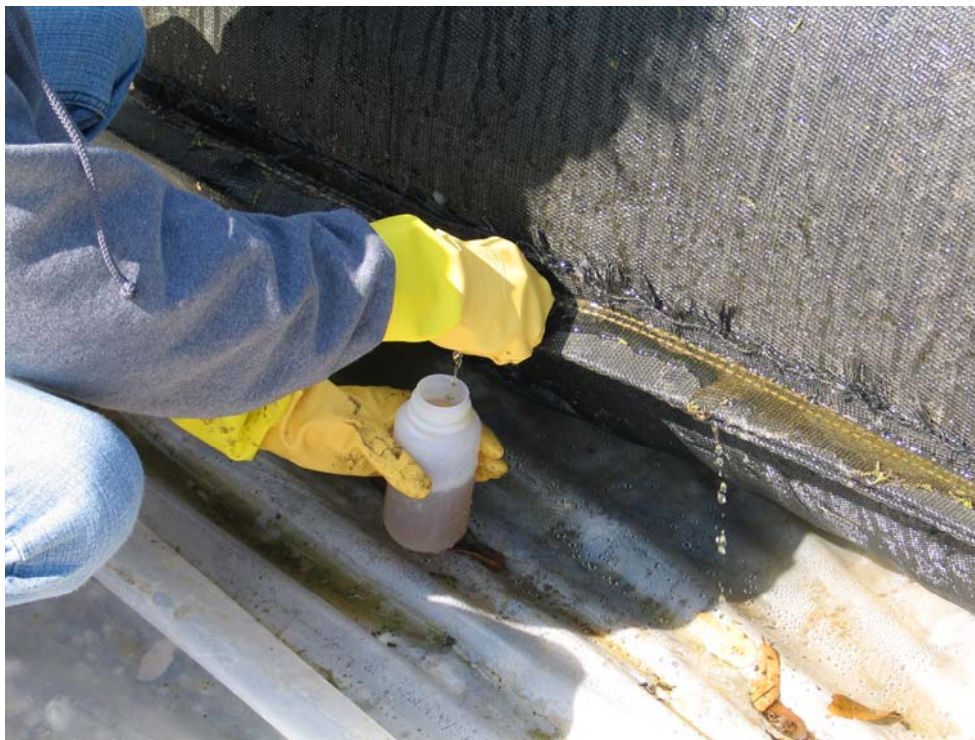
Figure 2. Collection of samples from Geotube Technology.
