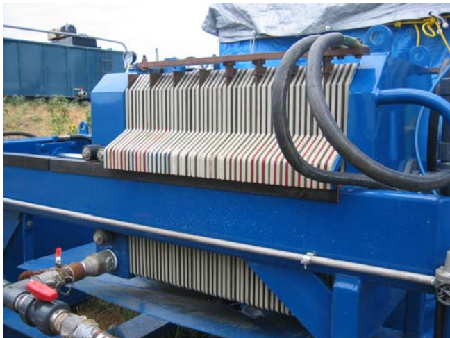
Figure 1. EC Unit: built on a filter press frame.
