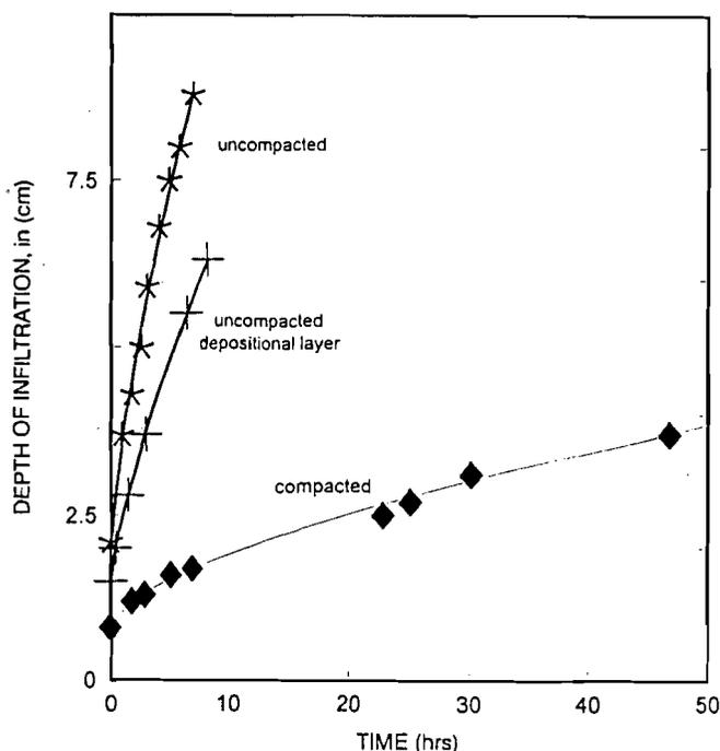
Figure 5. The depth of water penetration into alluvial soils after soil compaction to cause 5 mm of settling or the use of irrigation water containing suspended solids to make a 2 mm layer of deposition (Miyamoto, 1989).
