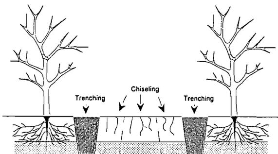
Figure 4. A sketch of a trench treatment used to improve stratified clay soils.
