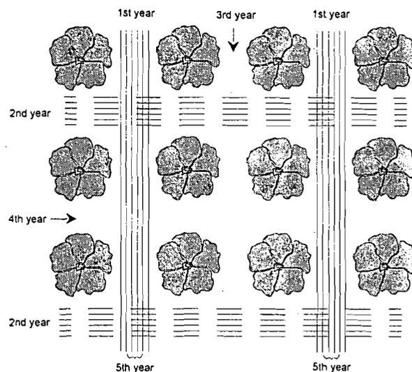
Figure 6. A system of soil chiseling implemented in a 4 year cycle. A new round of chiseling begins at the 5th year with a reduced width of chiseling strips.
