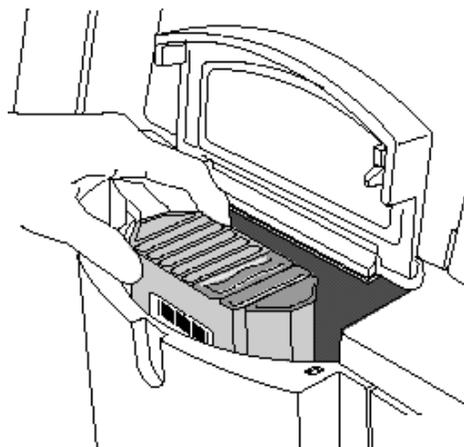
**CAUTION!** Push each insert firmly into place. If part of the insert extends above the top of the base, it could catch on the bottom of the deck and cause a system error. You could lose one or more batches as a result. Each insert is keyed by shape and cannot be inserted incorrectly.
