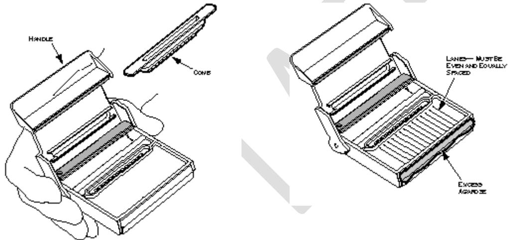
**Warning!** If the cassette shows a build up of excess gel on the front edge, or if you notice any shrinkage of the gel away from the cassette or bubbles, record the lot number and call Customer Support. Use a new cassette for this run.
