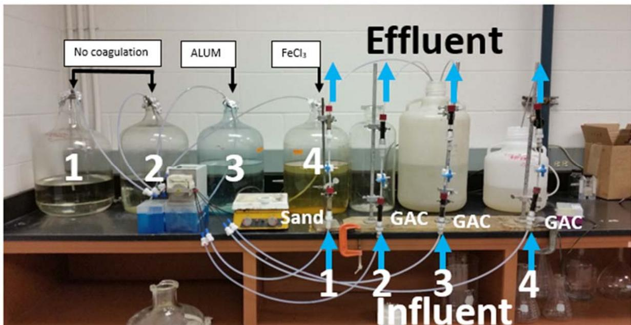
Figure 1. Bench-scale biofilter setup.
