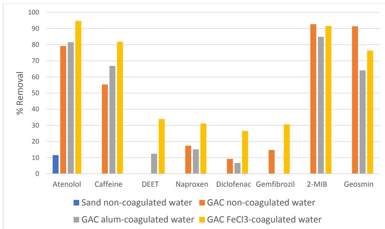
Figure 3. GC-MS and LC-MS/MS data for TrOC removal in the biofilter trains (6 months after start up). Each train was fed synthetic water with 0.5 µg/L of each TrOC.
