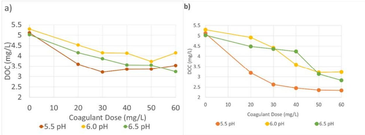
Figure 2. Jar test results for (a) alum and (b) ferric chloride coagulation.
