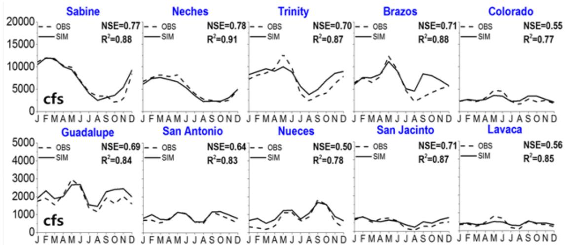
Figure 2. Monthly Calibrated (SIM) and Observed (OBS) streamflow (1960-1985)
