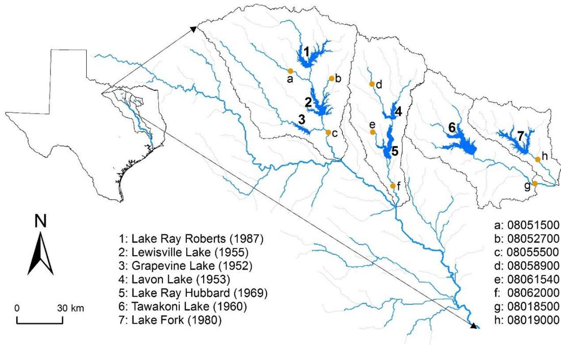
Figure 1. Dallas water source reservoirs and USGS streamflow gauges used for model calibration and validation.
