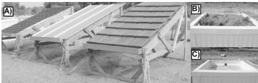
Figure 1. Pilot-scale roofs. (A) asphalt fiberglass shingle, Galvalume®, concrete tile; (B) green; (C) cool.
