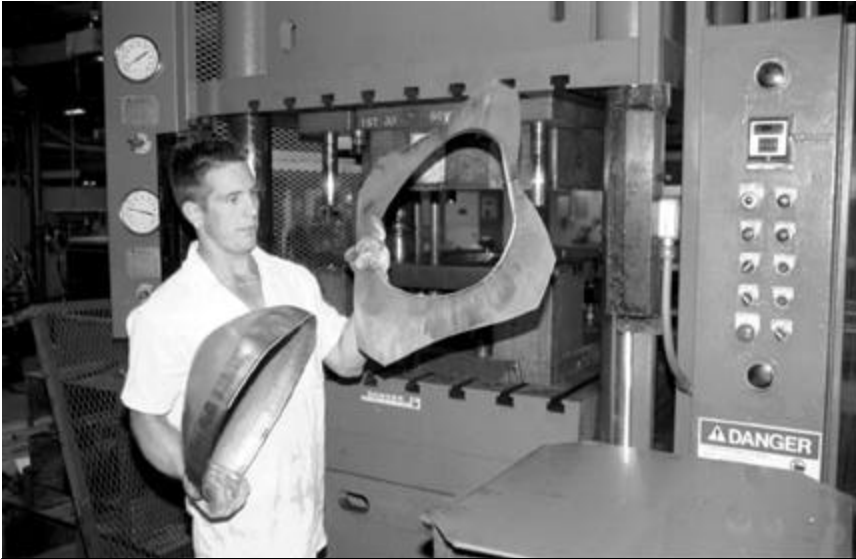
Workers at the TDCJ facility in Navasota manufacture water-conserving toilets specifically designed for use in prisons. Workers first build individual components including bowls (see photo, below), and then assemble the finished units (see photo, above).
