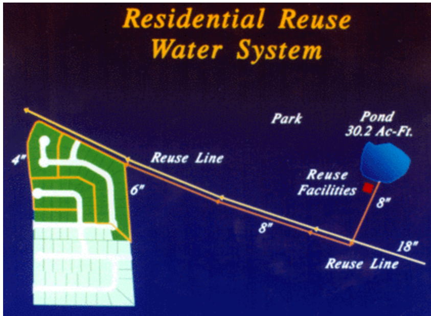
Schematic showing plans for a double water line system to allow for wastewater reuse for non-potable purposes in a residential setting.
