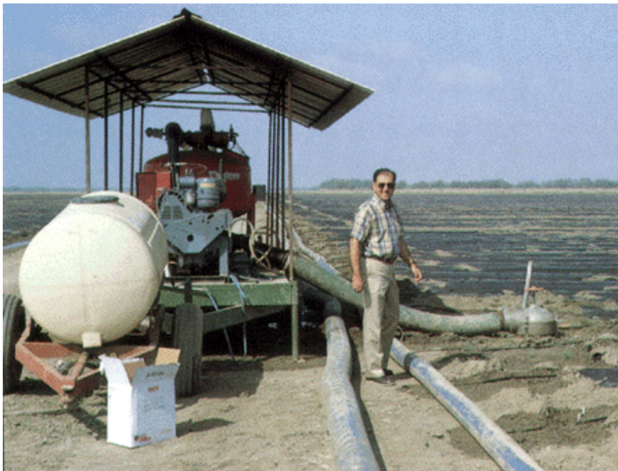
A portable drip irrigation trailer, shown here with Starr County Extension Agent Enrique Perez, delivers filtered pressurized water through tape-type tubing buried in melon field beds. The beds are covered with plastic mulch to reduce evaporation from the soil and prevent weed growth.
