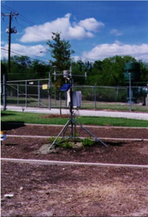
This weather station at the SAWS Jones-Maltsberger pumping station in north-central San Antonio collects data from which ET rates are calculated.
