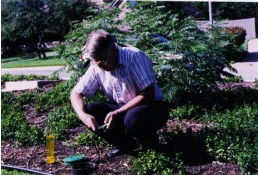
Wilber Watje, Bexar County Master Gardener and volunteer monitor for the San Antonio Pilot Evapotranspiration Study, checks soil moisture with an inductive sensor.
