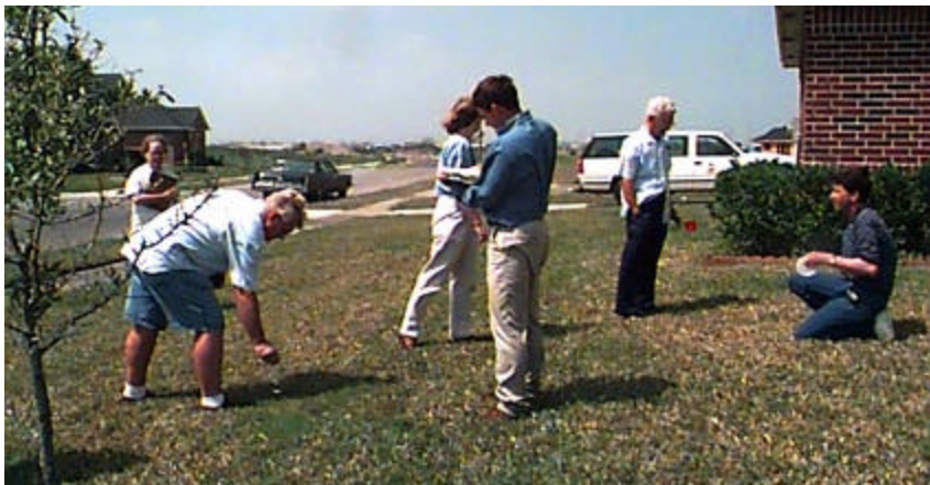
Master Gardeners remove catch-cans on a residential landscape after a 15-minute sprinkler irrigation test. Irrigation and Water Conservation Specialist David Smith records data, averaging the amount in all containers to determine sprinkler output
