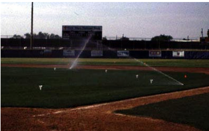
Catch cans allow irrigation auditors to quantify sprinkler output, as on this baseball field in Midway. In the School Athletic Field Education course, athletic field managers learn to adjust water use to be in concert with turfgrass requirements. Pesticide and fertilizer use is also addressed in the course.
