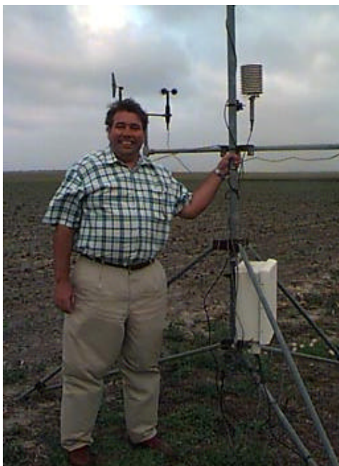
Juan Landivar, an agronomist at the Texas Agricultural Research and Extension Center in Corpus Christi, stands before a weather station which transmits climatological data to a central computer for computation of potential evapotranspiration.
