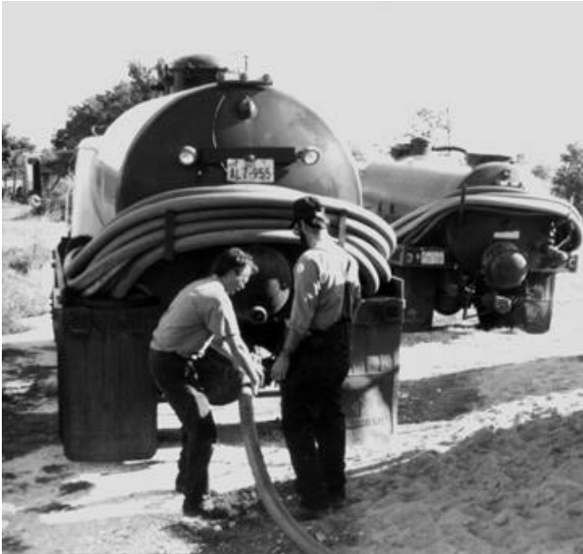
Domestic septage from the Austin area was delivered to the research site in Manor, TX (just east of Austin). The septage was dewatered, filtered, and blended with wood chips to produce compost.
