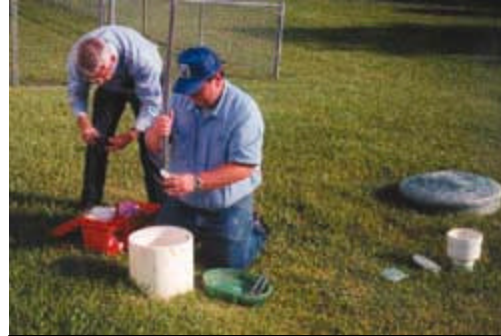
Staff members of the Trinity River Authority collect an effluent sample from this aerobic system near Lake Livingston.
