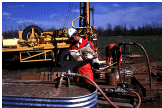
Part of the project involves using a device that sends heat impulses into the ground so that 3-dimensional groundwater flow patterns can be traced.
