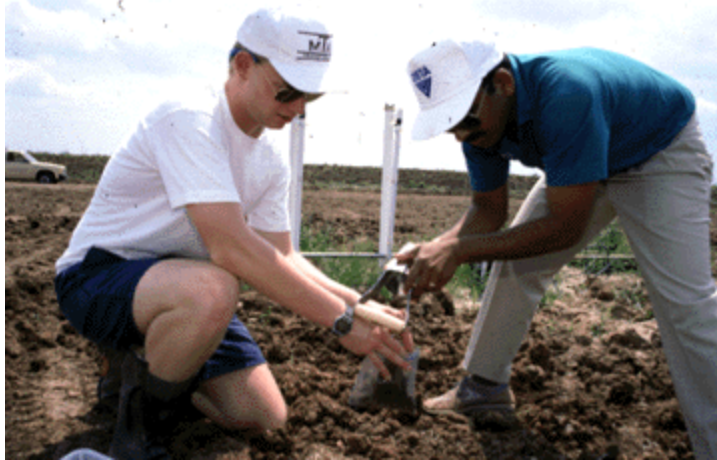
Texas A&M students install sensors in the ground that will automatically collect information on water levels and water quality.
