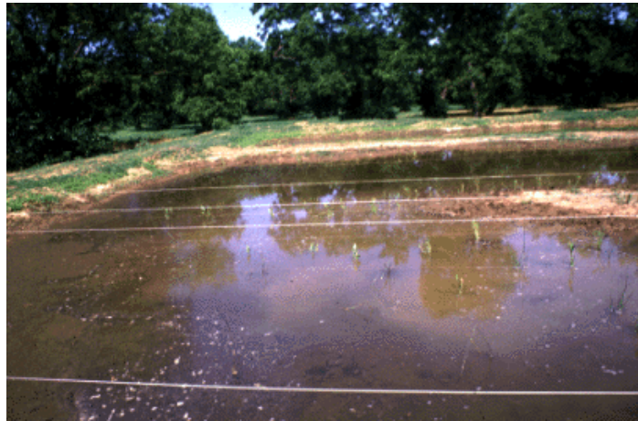
This experimental wetlands is being used to determine if it can remove pollutants and pesticides from runoff water.
