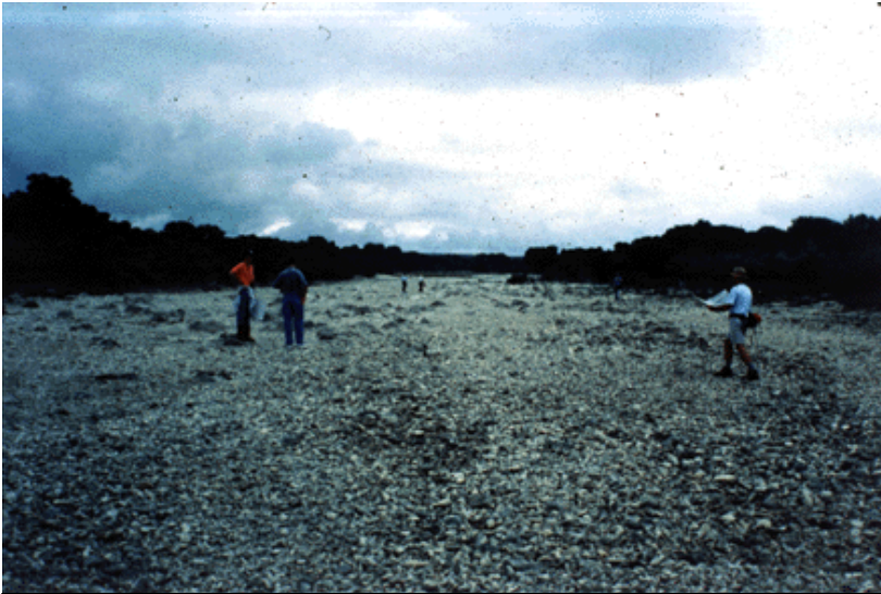
HDR engineers gathered field data from the Frio River (above) and other sites to assess channel losses.
