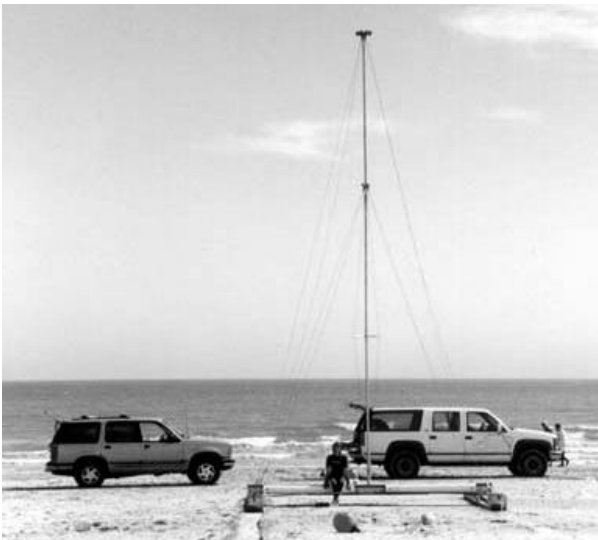
Researchers at Texas A&M University - Corpus Christi used this sea sled to conduct a survey of the beach bottom at South Padre Island. This unique device has two, 16-foot long runners and is towed along the beach bottom by a boat. It has a 40-foot high adjustable mast so surveys can be taken in deep waters.
