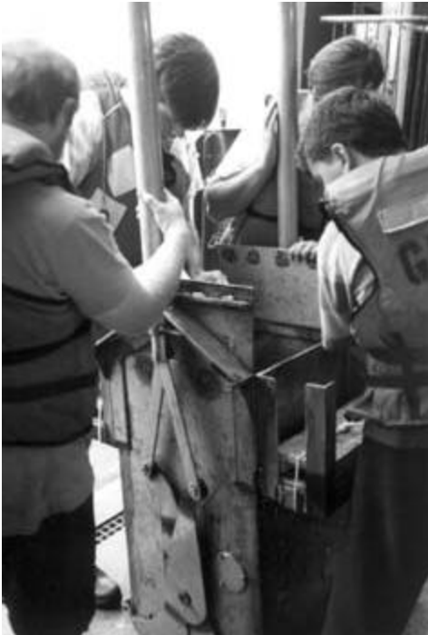
Texas A&M University-Galveston researchers on the research ship "Gyre" use this box corer to sample sediments..
