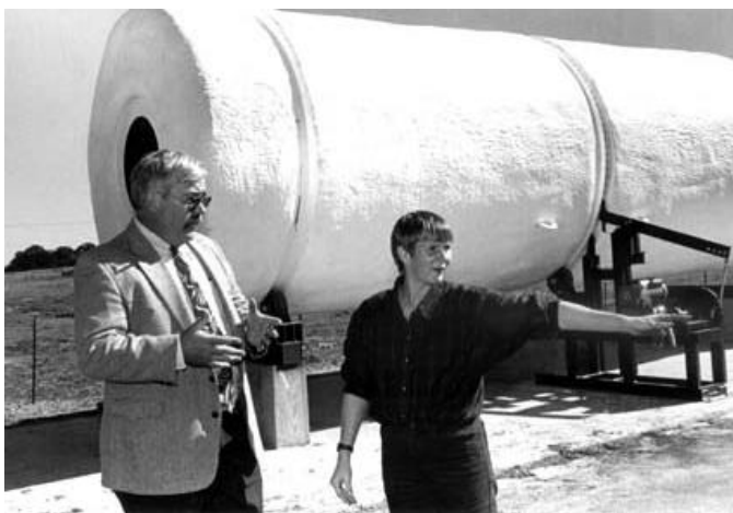
Don Cawthon of ETSU and Roelie Vellenga of Vellenga Dairies in Como, TX discuss the performance of this experimental composter. This device will be used to convert municipal sludge into a compost product that can be a substitute for peat moss.
