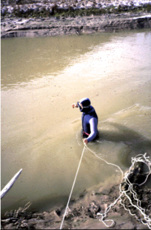
TWDB staff member Barry Hibbs collects this water quality sample on the Rio Grande. The goal of the project was to identify sources of total dissolved solids and salinity that flow into the Rio Grande alluvial aquifer.
