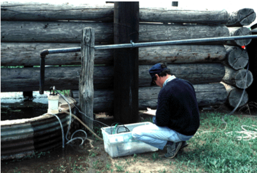
UT Research Assistant Steve Allen monitors this well near the Pantex Plant for salinity and pH levels.
