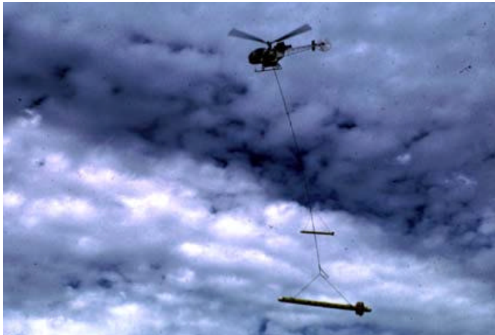
LCRA is using airborne electromagnetic surveying to detect the location of leaking oil wells.
