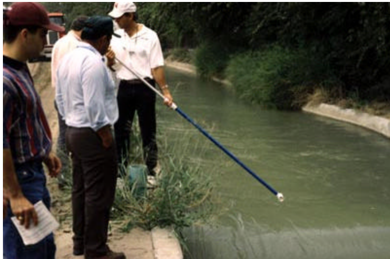
Steve Driewer prepares to measure the velocity of water movement in this canal near Edinburg.
