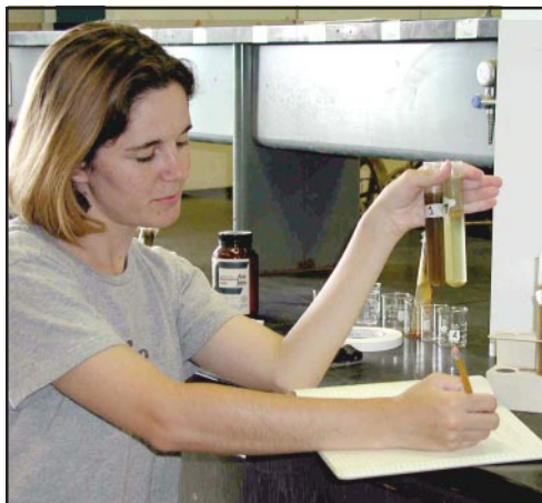
Photo courtesy of Amanda Bragg/ TAMU Amanda Bragg carries out a laboratory test to see how to precipitate phosphorus out of dairy wastewater.
