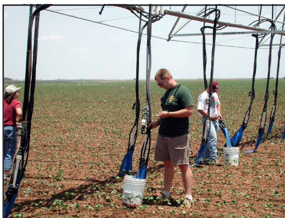
Photo by James Bordovsky/ TAES Stacey Ontai, Robert Stanaland, and Andrew Hurt check the flow rates of this LEPA irrigation system.
