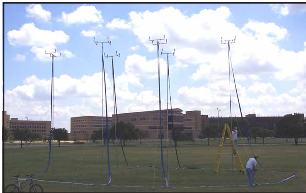
Photo Courtesy of Clyde Munster/ TAMU Students field test this rainfall simulator on the Texas A&M campus.
