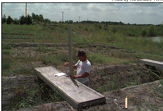
Tim Tucker of the Texas Transportation Institute measures the flow of water through this culvert at the
