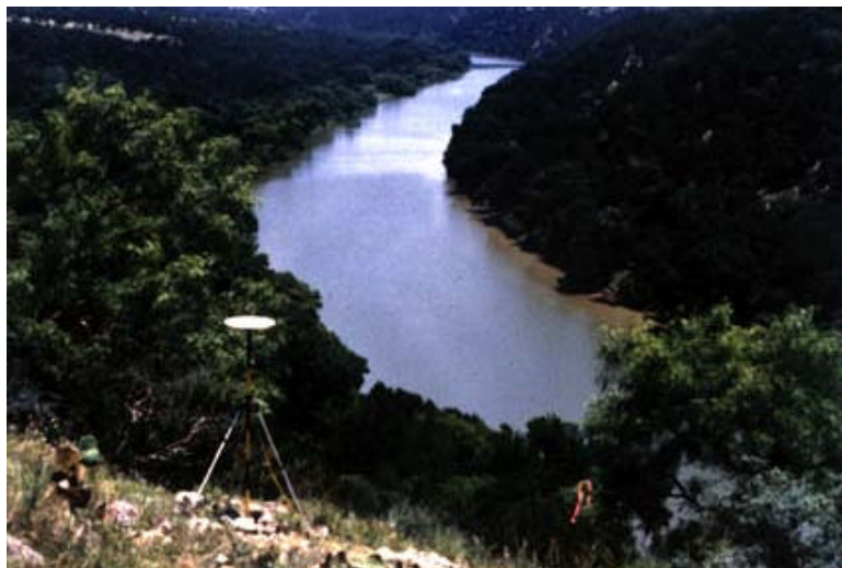
The LCRA uses benchmark stations like this one to properly orient the position of global positioning systems [GPS] that will be used during lake surveys. For example, these benchmarks [usually permanent positions near a lake] are located at a set of known coordinates. These benchmarks serve as reference points and help make sure that data obtained by GPS is accurate.
