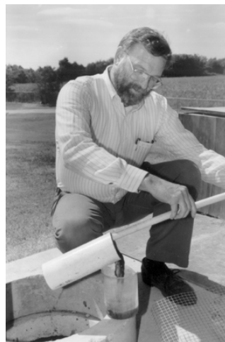
Dudley Burton of Baylor University gathers a water quality sample to see how well an aerobic on-site wastewater system provides treatment.
