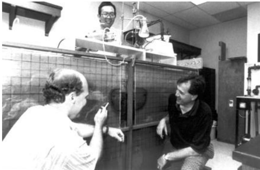
Mike Stallard (left) and Yavuz Corapcioglu (right) are examining this groundwater simulation tank to determine if levels of nitrate are being reduced. The goal is to develop a system that can remove nitrates from wells used for drinking water.
