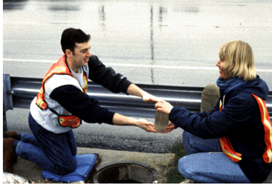
UT student Jeff Peters and UT CRWR research assistant Hanne Nielsen collect this water quality sample from Loop 1. These samples often contained oil and gas products and other automotive wastes.
