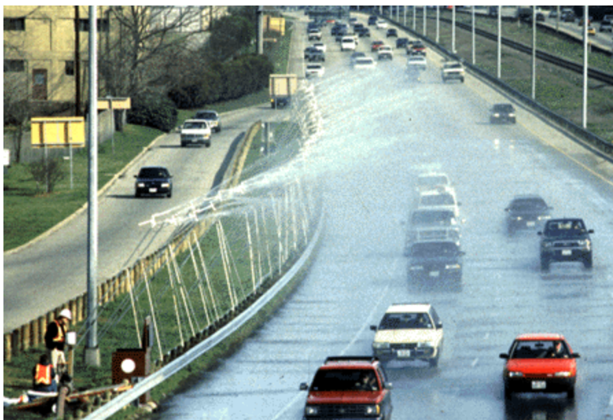
This rainfall simulator sprays precipitation onto Loop 1 in Austin. This was part of a research project at the Center for Research in Water Resources (CRWR) at UT Austin. The goal was to provide insights into the amount of pollutants carried by highway runoff and ways to treat that pollution.
