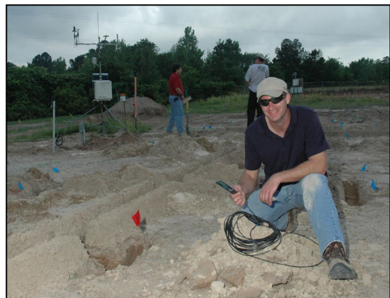
Dr. Karl Steddom, Texas AgriLife Extension Service plant pathologist, installs a moisture sensor at an irrigation test plot. (Texas AgriLife Extension Service photo by Robert Burns)
