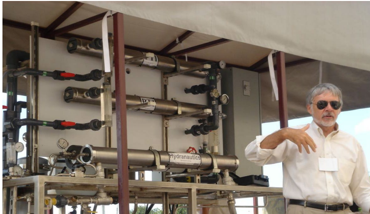
Dr. David Burnett , director of technology at the A&M System's Global Petroleum Research Institute, describes the mobile reverse-osmosis desalinator during a demonstration at the workshop in College Station.
