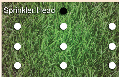
This grid shows placement of catch cans in relation to a sprinkler head.
