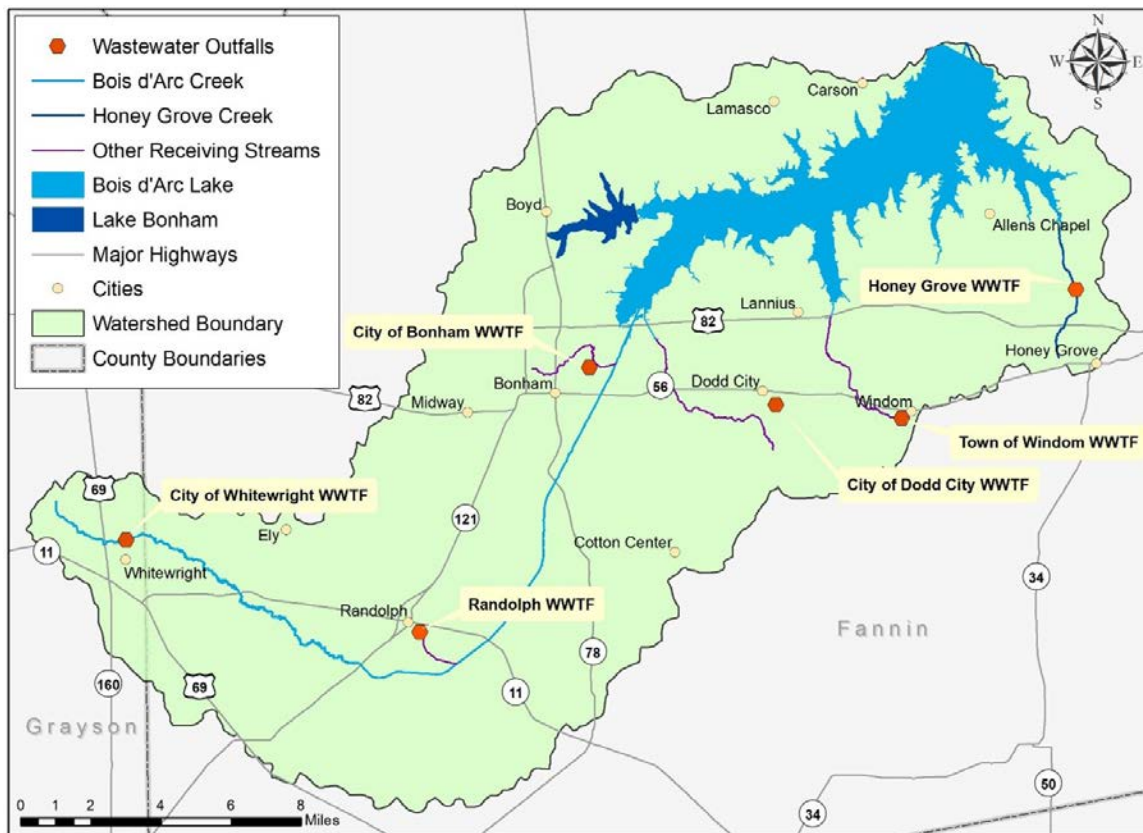
Figure 20. Active permitted wastewater discharge outfall locations for the Bois d'Arc Lake watershed.
