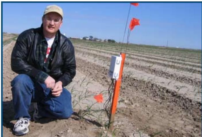
*Dr. Shad D. Nelson, associate professor of agronomy and horticulture at Texas A&M University-Kingsville, monitors water depletion in an ADI grower's drip irrigated onion field using real-time ECH2O EC-10 soil moisture sensors and automatic Em50 data loggers manufactured by Decagon Devices, Inc.*
