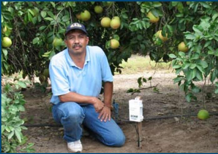
*Eddie Esquivel, ADI project coordinator, installs and monitors ECH2O probe soil moisture sensing and data logging equipment from Decagon Devices, Inc. beneath the canopy of microjet spray irrigated Rio Red grapefruit in an ADI collaborator's orchard.*
