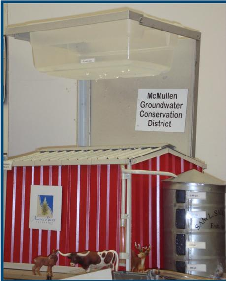
A mock-up of a rainwater harvesting system was displayed at the Uvalde workshop by Nueces River Authority. This system simulates rainfall so participants can visually see the rainwater being captured.
