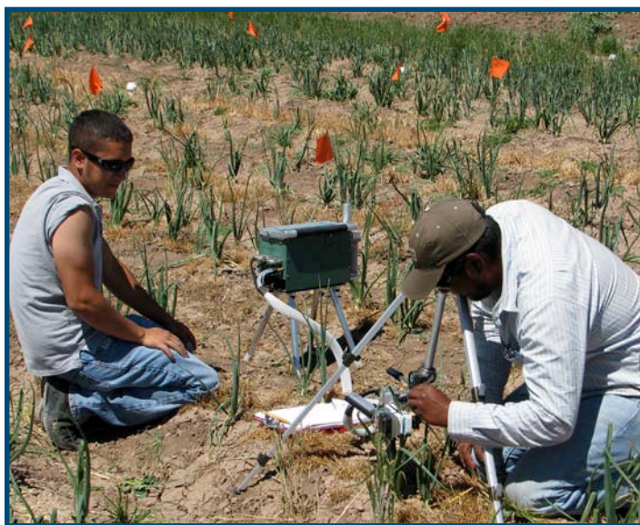
Graduate student Tony Rios (right) and agronomy undergraduate Samuel Diaz (left) adjust the leaf chamber used to measure plant gas exchange in onions. Data collected in this experiment was used to quantify plant stress, photosynthesis rates, and water use efficiency.
