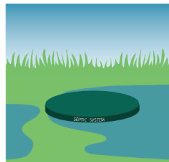
Standing water or damp spots near your septic tank or drainfield/sprayfield
