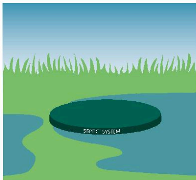
Standing water or damp spots near your septic tank or drainfield/sprayfield
