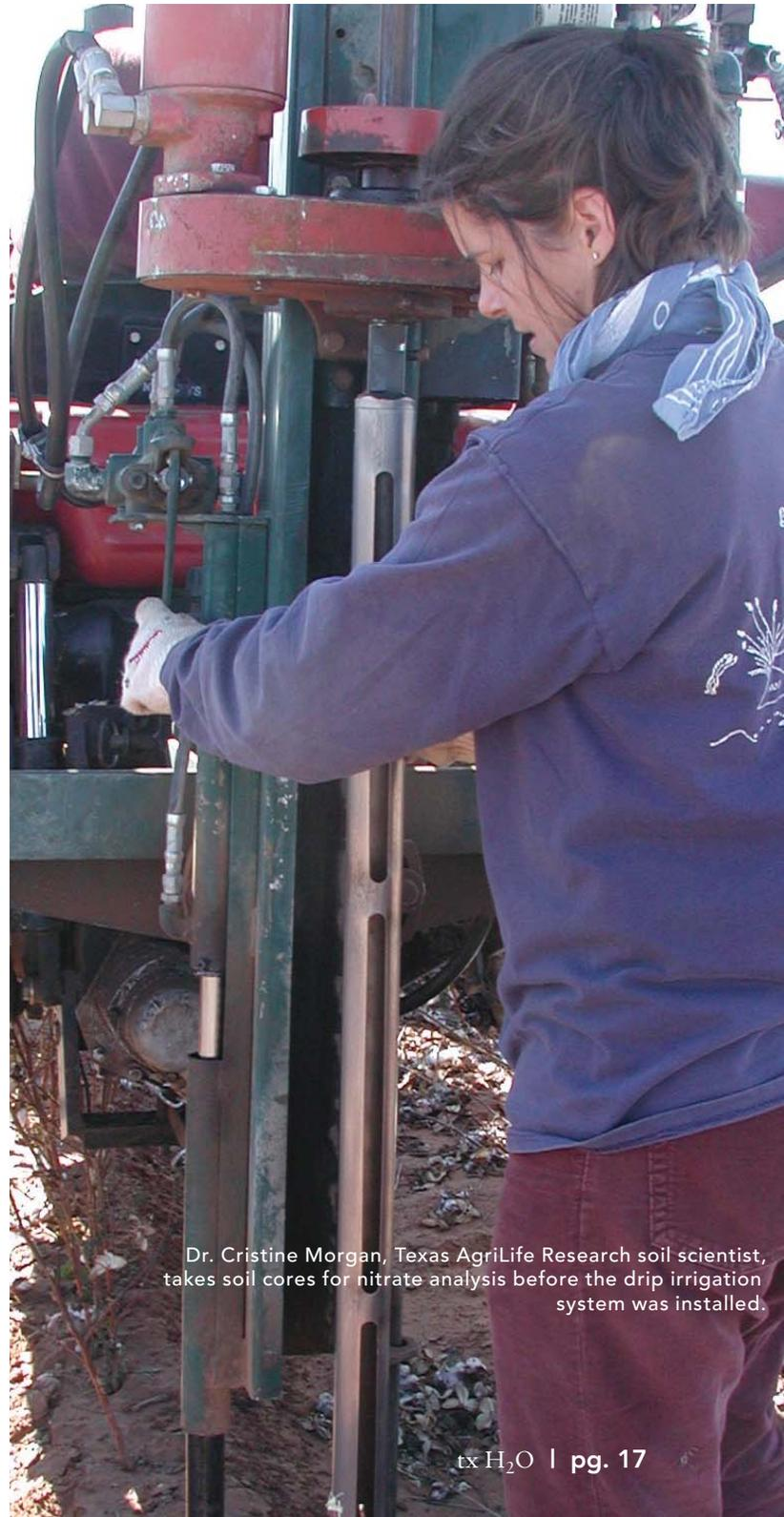
Dr. Cristine Morgan, Texas AgriLife Research soil scientist, takes soil cores for nitrate analysis before the drip irrigation system was installed.
