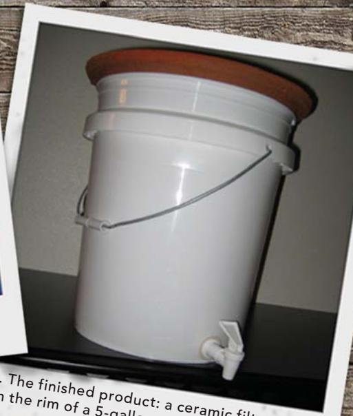
6. The finished product: a ceramic filter rests on the rim of a 5-gallon water container.
