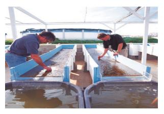
The research center consists of 12 manmade "streams" that imitate natural rivers found throughout the region. Each experimental stream is 16 feet long and two feet wide. To mimic real world conditions, the streams were built with a gravel substrate, and pools were placed at the end of each stream segment. Water is supplied by the wastewater plant. A variety of aquatic organisms (including insects, larvae, snails, invertebrates, and fish) was obtained from Pecan Creek for
