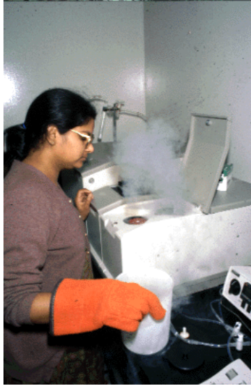
Research Associate Amita Jain prepares the Fourier transform infrared spectrometer for analysis of arsenic contaminated sediment samples. The infrared spectrometer is used in studies of arsenic binding to sediment colloids.
